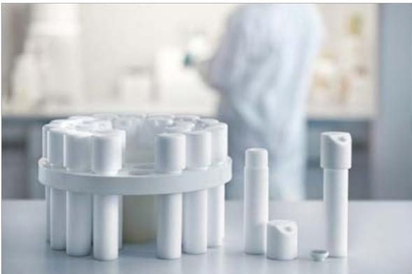
Pressure digestion vessels made of TFM™-PTFE
