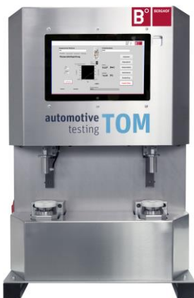
Membrane testing for water penetration and volume measurement
